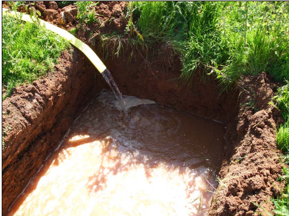
Figure 6: Undertaking an infiltration test in alluvial soils, UK.
